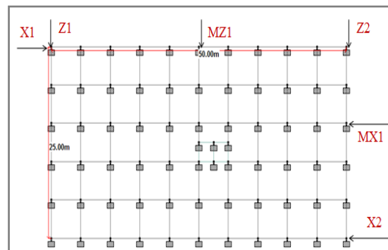
Fig. 2.1 Cases for building of lift core at centre
